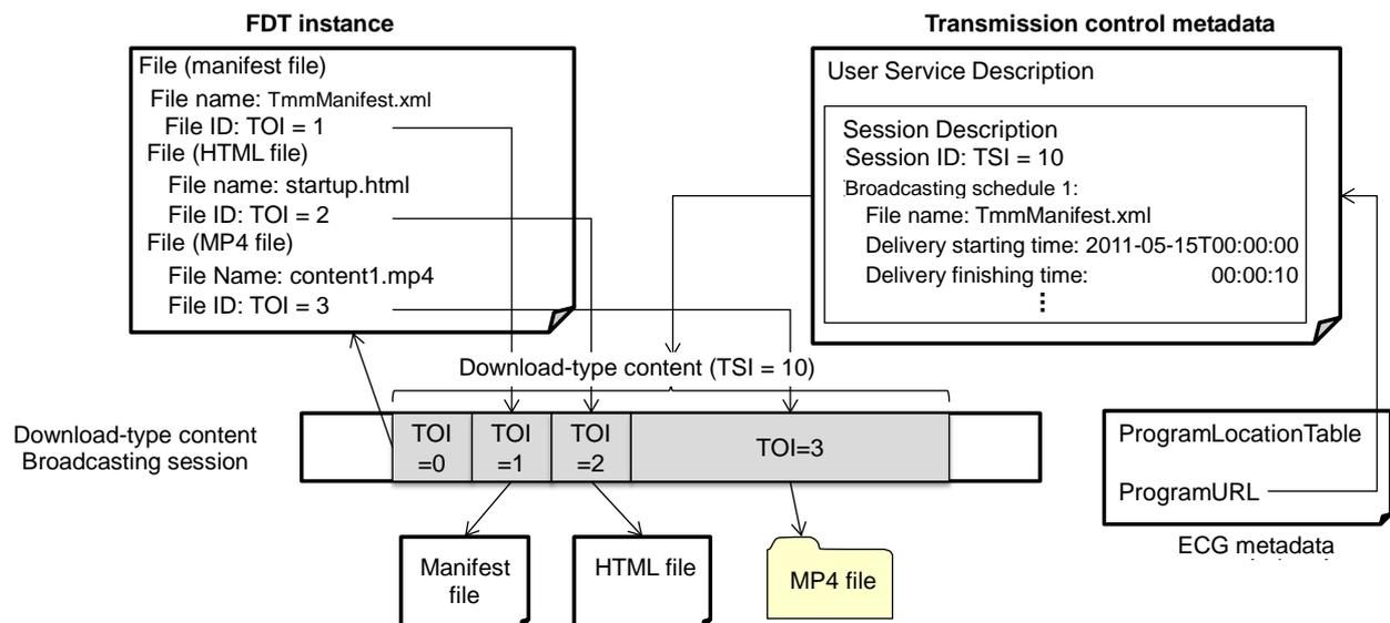
Fig. 6-5: Reference relationship between transmission control metadata and download-type content
