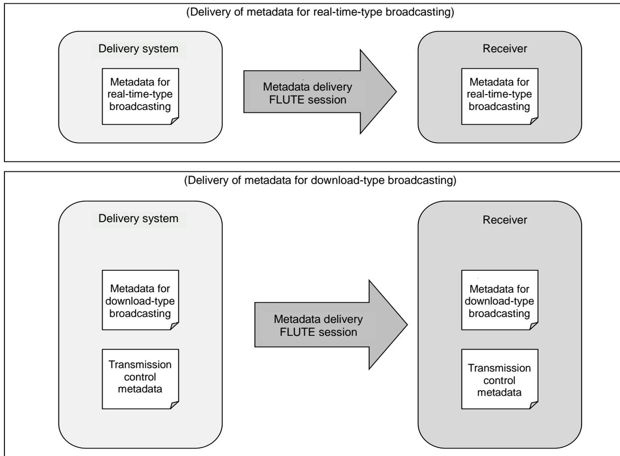
Fig. 6-2: Conceptual diagram for metadata delivery operation in metadata delivery system A
