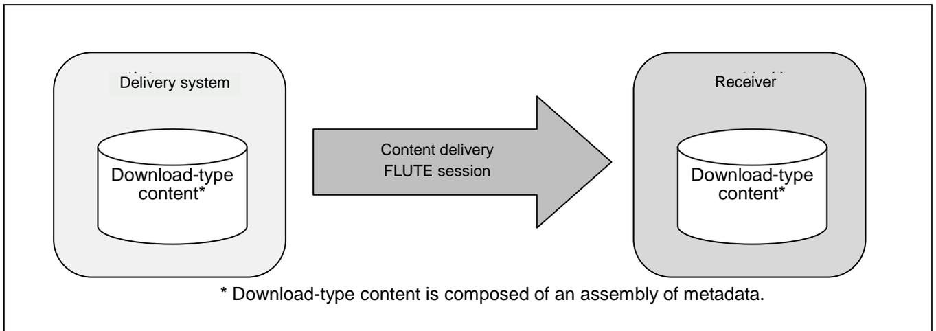
Fig. 6-3: Conceptual diagram for metadata delivery operation in metadata delivery system B
