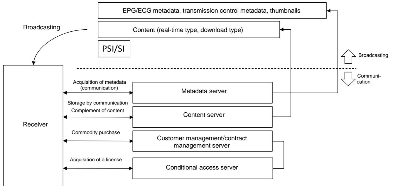
Fig. 3-2: Example of a typical server/receiver configuration involved in download-type broadcasting
