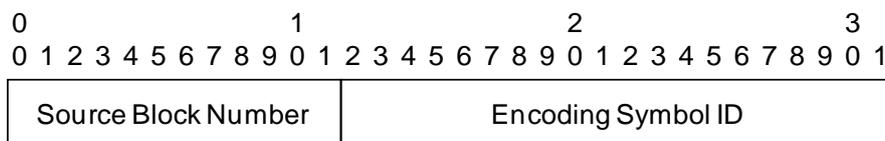
Fig. C-3: FEC Payload ID
