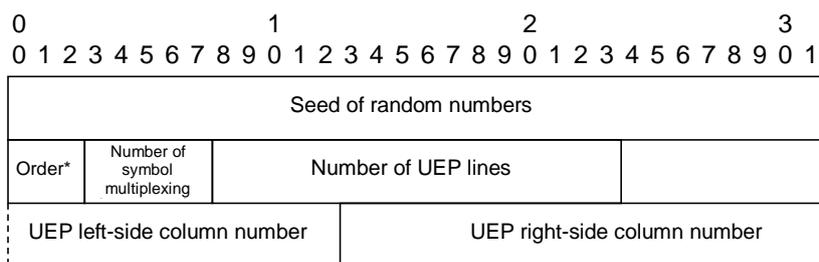
Fig. C-2: FEC-OTI-Scheme-Specific-Info (when UEP is in use)
