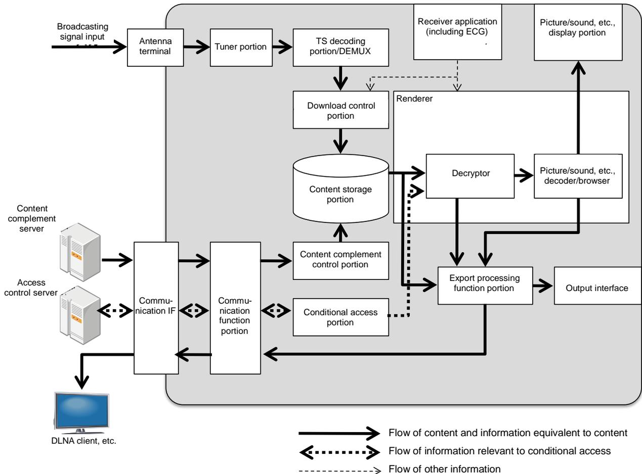
Fig. 3-1: Example of a typical receiver configuration involved in download-type broadcasting
