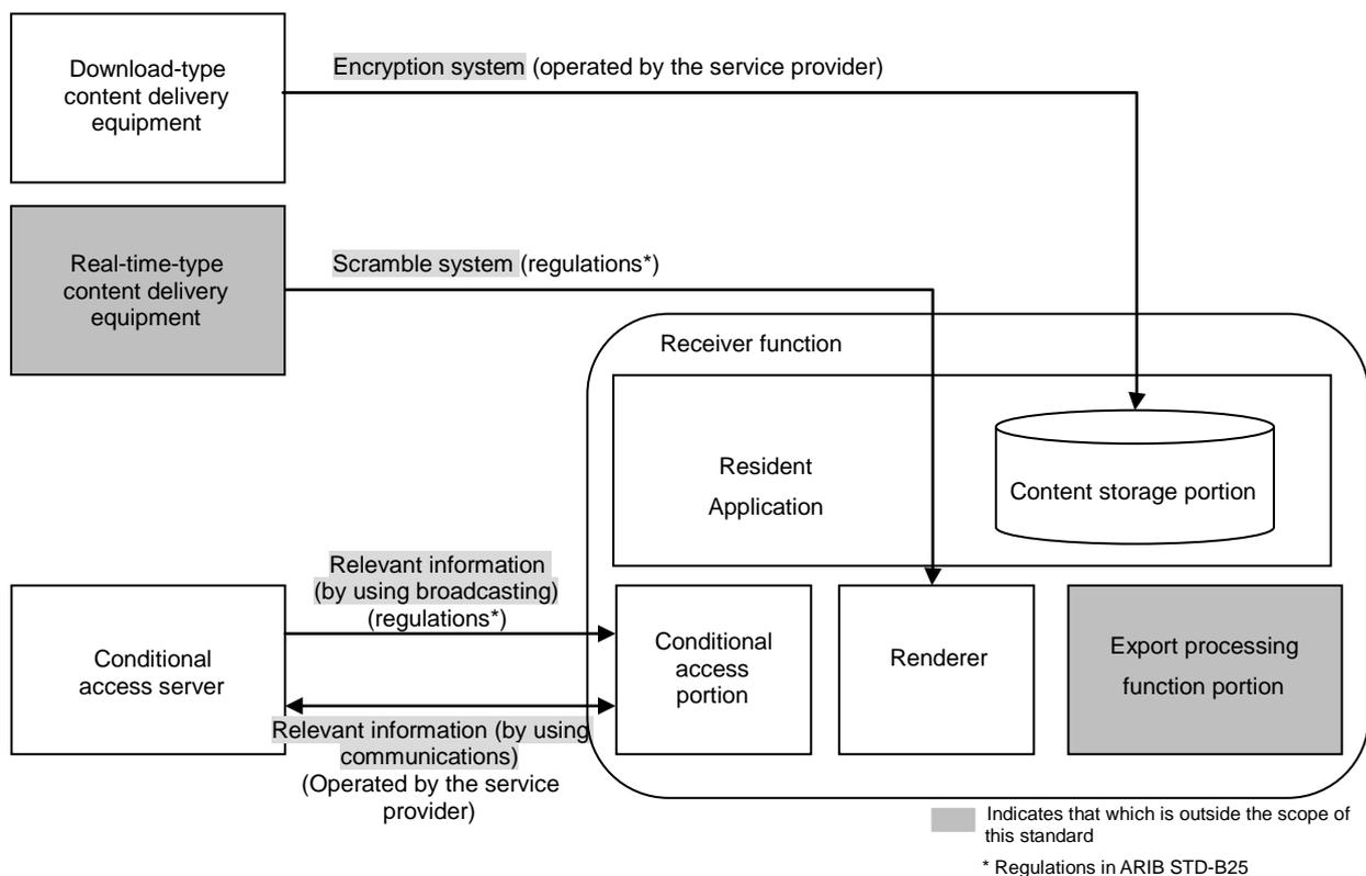
Fig. 4-1: Outline of the conditional access system involved in ISDB-Tmm terrestrial mobile multimedia broadcasting
