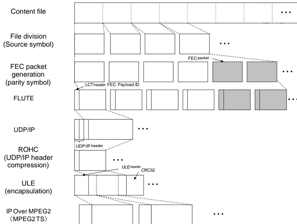
Fig. 8-1: Processing starting from a content file up to transmission by mpeg-2 ts
